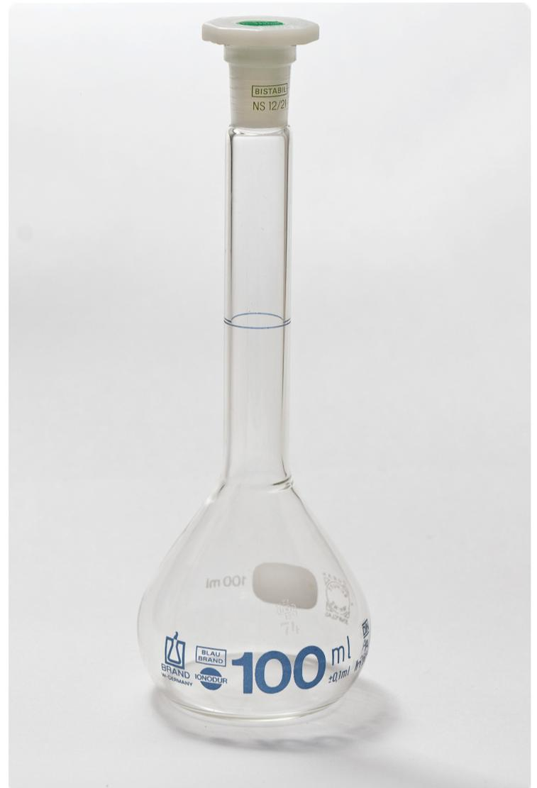
Figure 3.9: Volumetric Flask: "[File:Brand volumetric flask 100ml.jpg](#)" by [Lucasbosch](#) is licensed under [CC BY-SA 3.0](#).
