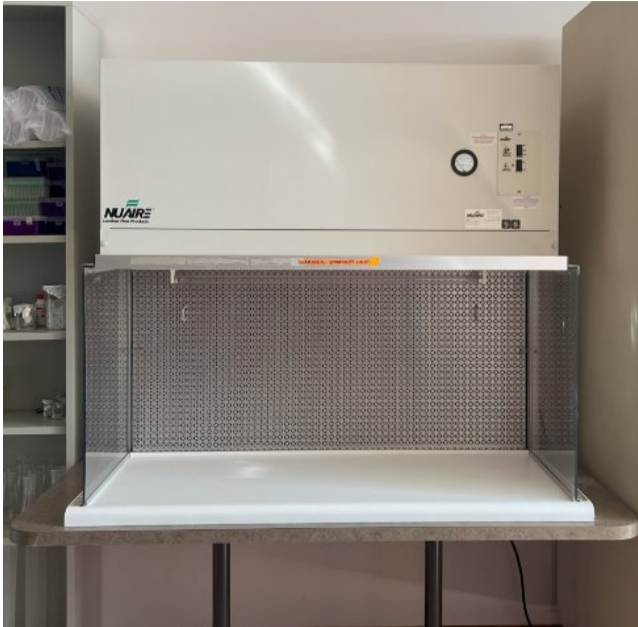
Figure 1.4 Laminar Flow Hood. Image by Author
